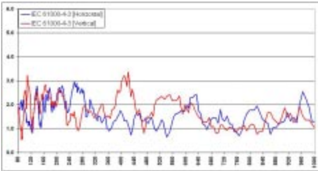
Measured Field Uniformity from 80 MHz to 1000 MHz
