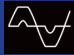
Oscilloscope of voltage and current waveform at load due to distribution losses. THD=6.6%
